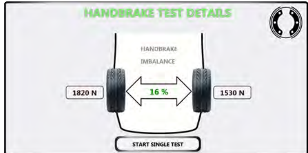
Measures: Left to right hand brake imbalance, for cable style handbrakes.
